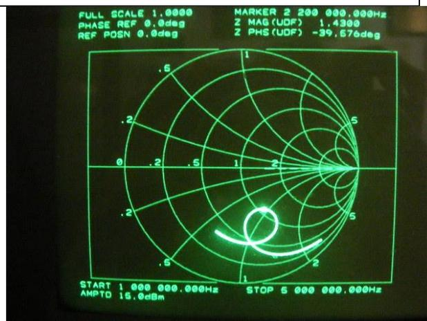
When 10 ft. of Cat-5 cable is inserted between the load and the source, at 2.2 Mhz, the impedance drops from 72 ohms to 56 ohms and the phase is shifted from -40 degrees to -26 degrees. This is still a little short of the 50 ohm resistive goal we are trying to reach.
