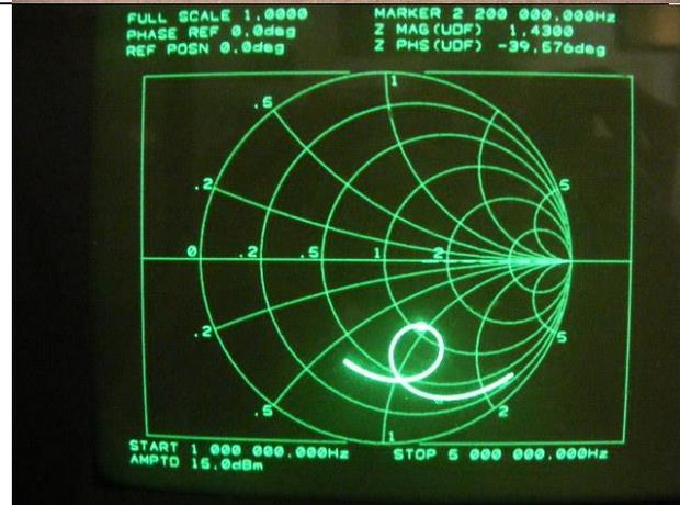
The Smith chart on the right contains a set of light green concentric lines. These are constant resistance lines. Inserting a standard value 3.9uH inductor in series with the modeled transducer load adds inductive reactance to the otherwise capacitive circuit without significantly changing the circuit's resistance.
