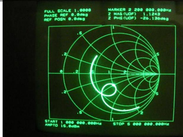
The load impedance seen by the source can be modified by adding an impedance matching circuit between the cable and the load. Inserting an L-pad matching network consisting of 2.2uH and 47uH, between the analyzer and the Cat-5 cable brings the 2.2 Mhz impedance measured at the source to 63 ohms and reduces the phase to 1 degree. This match, although not ideal, allows for some degradation of the transducer Q over the life of the device.
